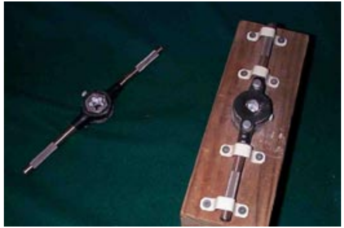
Photo of rod threader and rod threader mounted on 4x4 for straight alignment.
